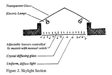
At the time of the design, electric lamps were a new technology. They were placed in the attic cavity to reinforce and augment the daylight. This approach allowed the design to avoid having the electric light sources located within the galleries as additional objects. The hidden locations were determined to best light the displays and avoid the creation of hot spots on the ceiling.
